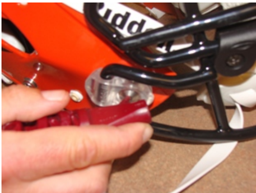
Speed Release Clamp (Use special tool or ball point pen to release) *Do NOT use spring loaded window punch
